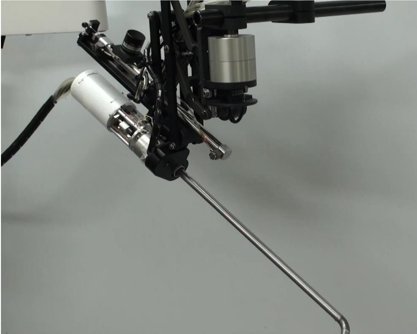
RCM-type surgical robot prototype developed in Tokyo Institute of Technology
